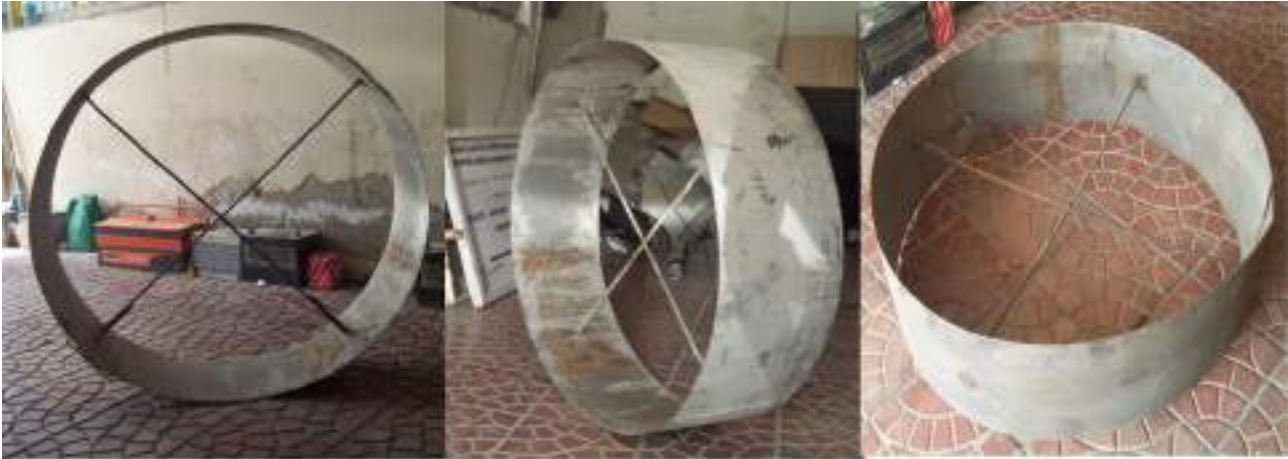
Figure 5: mold for pit lining
