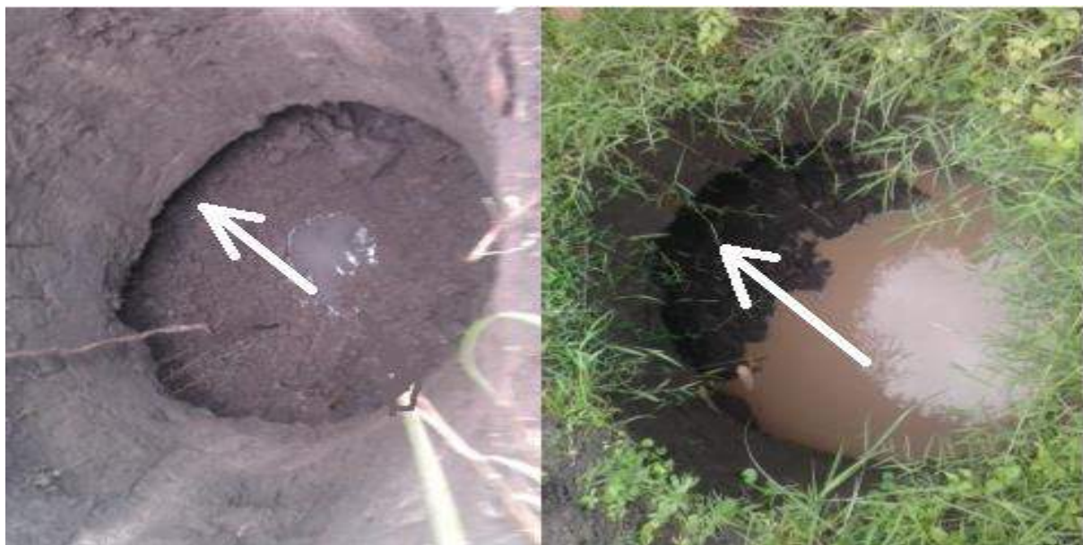
Figure 2: How pit collapse happens
