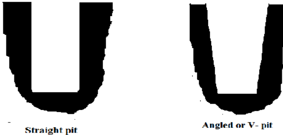
Figure 3: pit with different shapes
