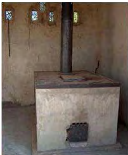
Fig. 9: Medical waste incinerator constructed on the Health Center's compound, 2004 (source: EcoSan Club)
