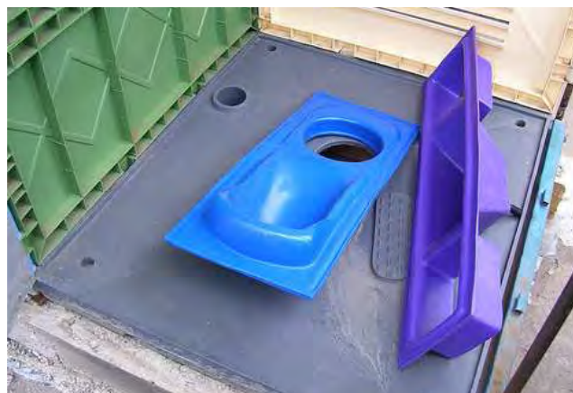
Fig. 10: Various urine diversion plates at the factory of Kentainer. The double vault plate was developed by EPP (source: C.Rieck, GIZ-Kenya, Jan 2010).
