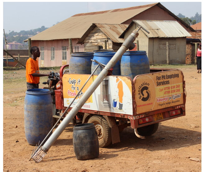
Gulping Pit emptying technology
