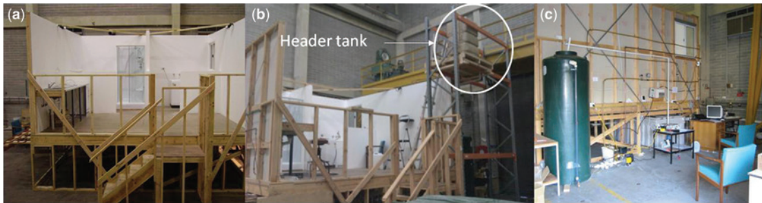
Figure 6.16 Simulated dwelling for evaluation of energy use for rainwater supply (a) Overview of major end uses (washing machine, toilet, taps and dishwasher), (b) Set-up for rainwater supply with a 300 litre header tank, (c) Rainwater tank supply and monitoring instrumentation.
