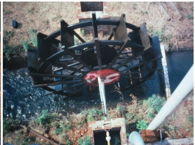
The writer and his pump in 1979. On the right a photo taken from the 8m tower looking down on the pump. The principle was first discovered by a Mr A Wirtz and his invention of 1746, but appears to have been lost to science. This work drew attention back to this novel concept.
