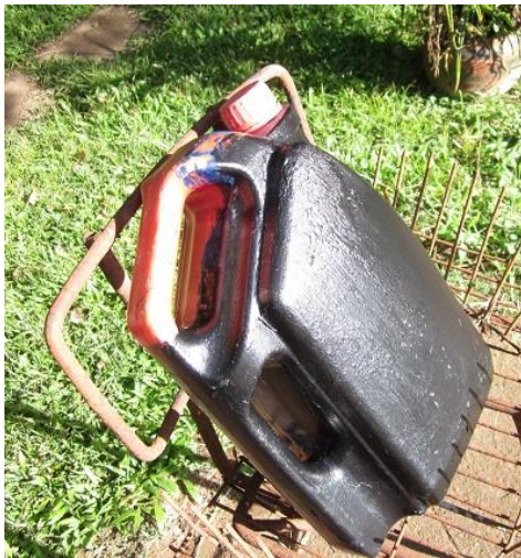
Left: simple solar water heater made from a used 5 litres plastic oil container and painted black on one side. It is placed at a slant to face the sun. The slant also produced a circulation of water within the container. Middle: The shower unit is simply made from a bucket and pipe fittings and can hold about 9 litres of heated water. The water can be heated by the sun, gas or electricity. It makes an excellent shower. Right: the essential candle filter to purify water. This version was made in India, but the candles have been changed several times. The latest candles were made in the UK. The candle filter is an excellent way of purifying water bacteriologically.
