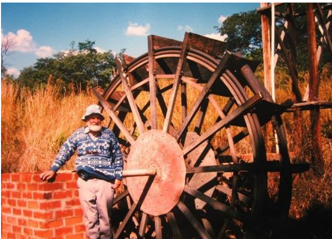
The writer and his pump in 1979. On the right a photo taken from the 8m tower looking down on the pump. The principle was first discovered by a Mr A Wirtz and his invention of 1746, but appears to have been lost to science. This work drew attention back to this novel concept.
