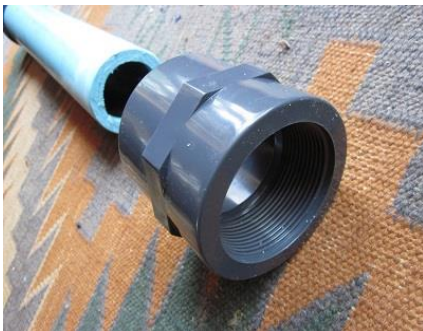
PVC inserts are bonded beneath the stainless steel cylinder pipe, as a means of holding the piston above the bottom of the cylinder tube. A standard 63mm to 2 inch PVC pipe adaptor is solvent cemented to the bottom of the cylinder. The brass foot valve is threaded into this fitting. The centre photo shows the upper end of the cylinder inside the PVC pipe. A standard PVC 63mm connector is then solvent cemented to the top of the cylinder pipe.
