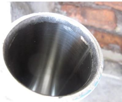
PVC inserts are bonded beneath the stainless steel cylinder pipe, as a means of holding the piston above the bottom of the cylinder tube. A standard 63mm to 2 inch PVC pipe adaptor is solvent cemented to the bottom of the cylinder. The brass foot valve is threaded into this fitting. The centre photo shows the upper end of the cylinder inside the PVC pipe. A standard PVC 63mm connector is then solvent cemented to the top of the cylinder pipe.
