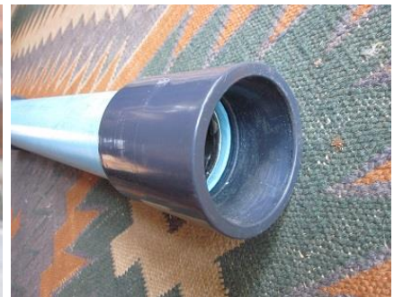
PVC inserts are bonded beneath the stainless steel cylinder pipe, as a means of holding the piston above the bottom of the cylinder tube. A standard 63mm to 2 inch PVC pipe adaptor is solvent cemented to the bottom of the cylinder. The brass foot valve is threaded into this fitting. The centre photo shows the upper end of the cylinder inside the PVC pipe. A standard PVC 63mm connector is then solvent cemented to the top of the cylinder pipe.
