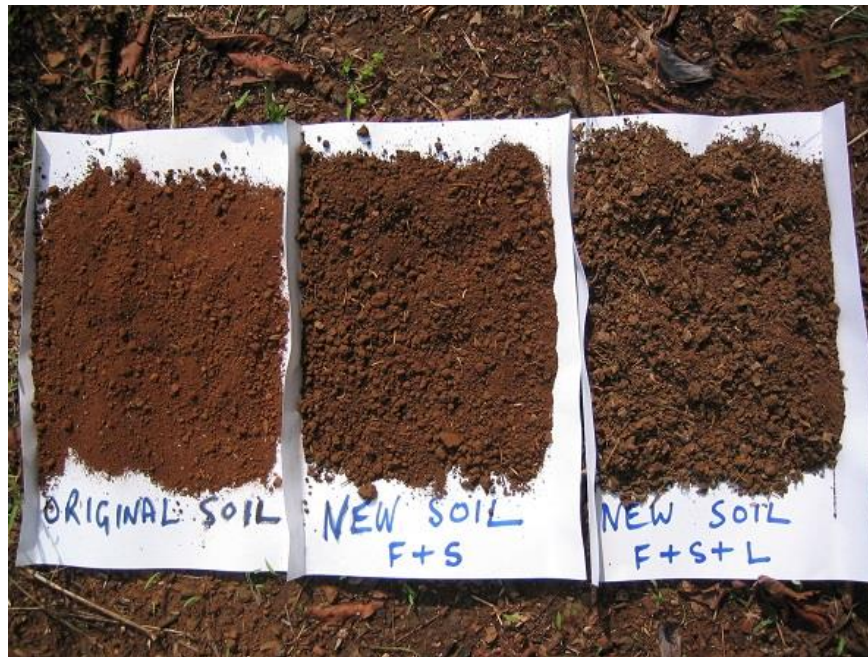
Samples of original soil (left), and “new soil” made from faeces and soil (centre) and from faeces, soil and leaves (right)
