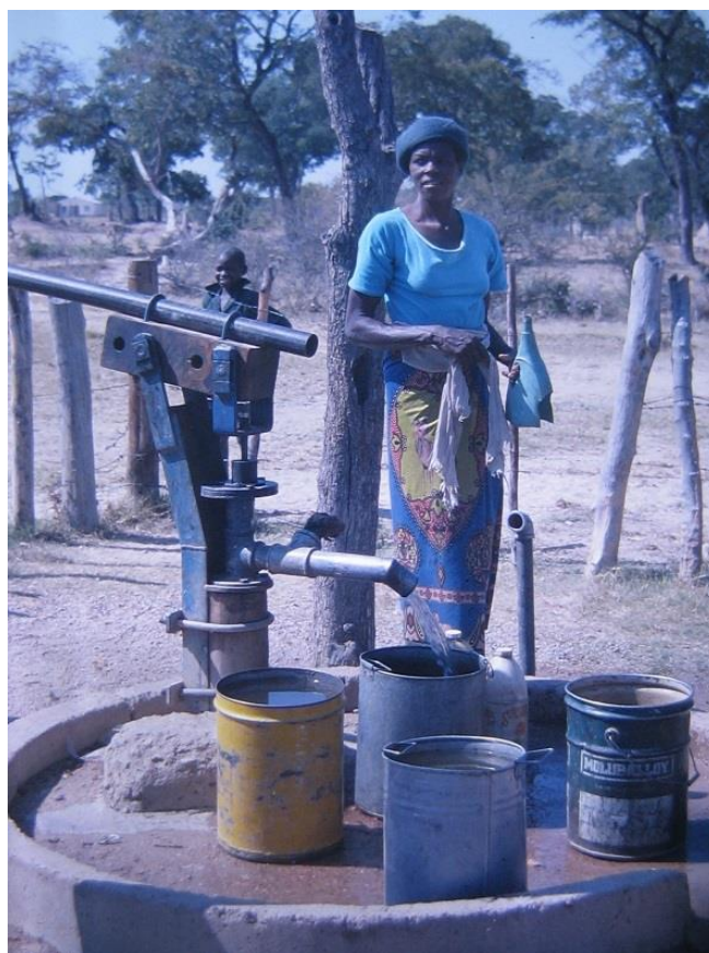
Left: The first B type Bush Pump being tested in Epworth, 1987. Right: A later B type Bush Pump being tested in the field by DDF.
