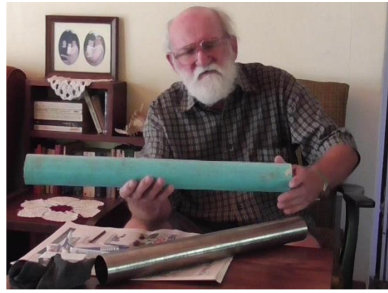
The stainless steel tube and the 63mm class 12 or 16 PVC pipe into which the tube is bonded. Details of the procedure of preparing the cylinder in its casing can be found on the DVD.
