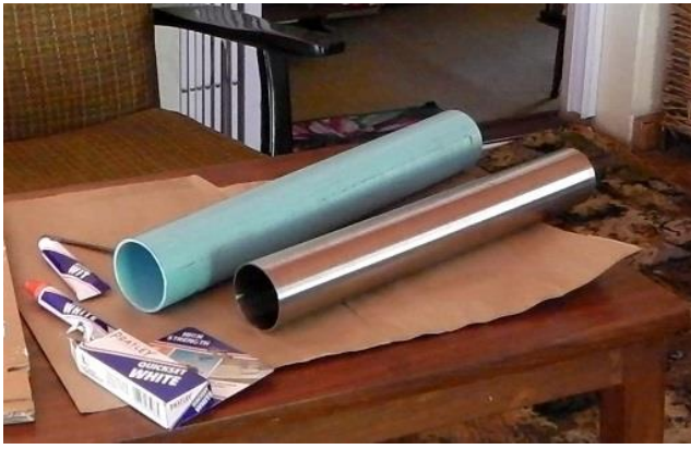
The stainless steel tube and the 63mm class 12 or 16 PVC pipe into which the tube is bonded. Details of the procedure of preparing the cylinder in its casing can be found on the DVD.
