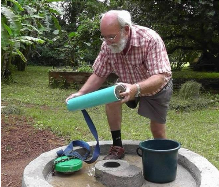
Making and testing a home-made bucket pump in the garden
