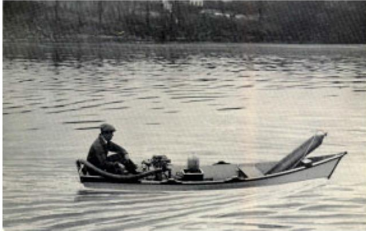
The W&T Chloro-boat was used for disinfecting large reservoirs or sterilizing large outdoor swimming areas.
