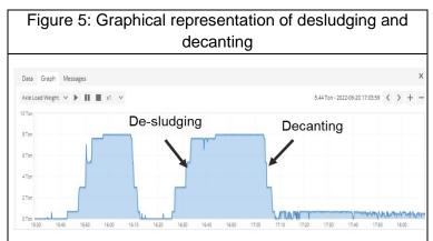
limb of the graph depicts the desludging of containment with increasing vehicle axle load and
