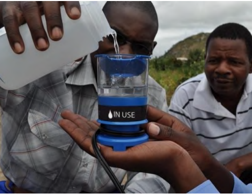
Figure 9. MSR SE200 community chlorine maker (Source: PATH)
