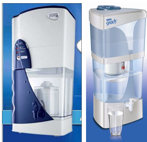
Figure 6: The Pureit (on the left) can be used to treat about 1500 liters of water (depending on the model) using a carbon block to absorb and filter impurities, followed by chlorine disinfection; replacement of the chlorine unit enables treatment of 1500 liters more. The Tata Swach (on the right) uses rice husk ash and silver to treat water; it enables treatment of up to 3000 liters before the so-called treatment “bulb” must be replaced.
