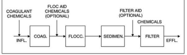
Figure 6 Schematic diagram of conventional filtration processes at Zomba and Liwonde water treatment plant. INFL-Influent, EFFL- Effluent, COAG- Coagulation, SEDIMEN- Sedimentation, FLOCC- Flocculation. Source (Manda, Chidya et al. 2016)
